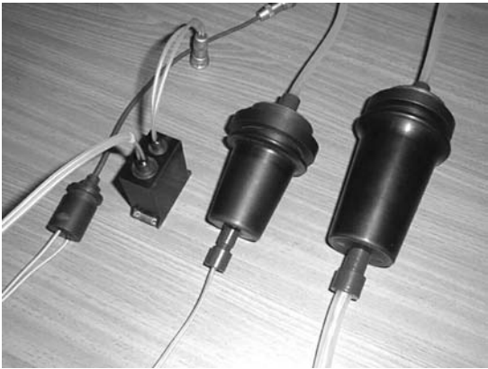
FIGURE 6.21 HV interface RG-series relays for industrial and military applications.
