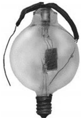
FIGURE 7.7 The first three-electrode vacuum tube constructed by Lee De Forest.
