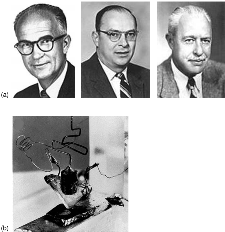
FIGURE 7.44 (a) Inventors of the transistor, the Nobel Prize laureates: William Bradford Shockley, John Bardeen, and Walter Houser Brattain. (b) This is how the first laboratory sample of a transistor looked.
