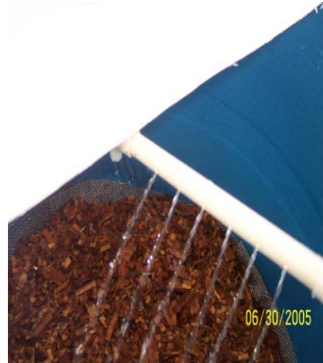
Figure 18: Liquid Sprays on Top of Chips
