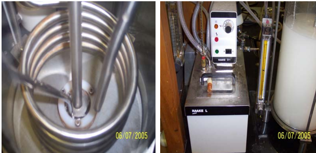
Figure 40: Cooling Coil Sit Above the Aerator Figure 41: Cooling Temperature Control
