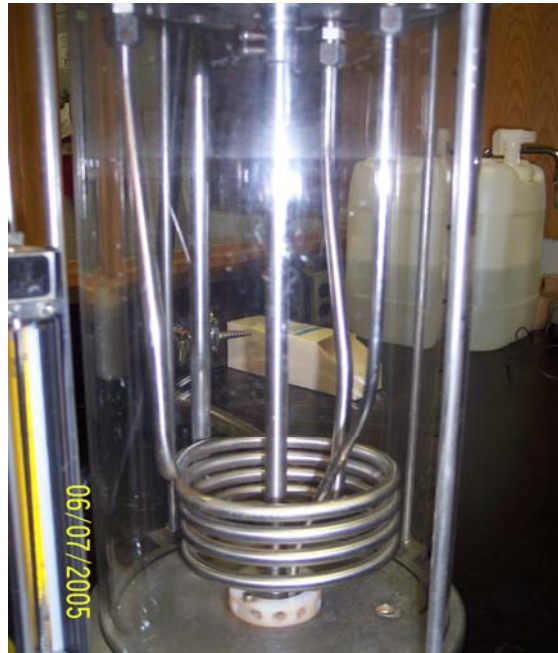
Figure 39: Cooling Coil in the Fermentor
