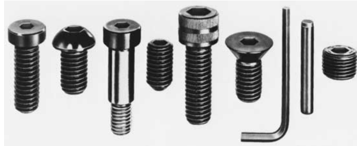
FIGURE 23.5 Hex-socket fasteners. From left to right, the parts are identified as a low socket-head cap screw, a button-head socket cap screw, a socket shoulder screw, a socket set screw, a socket-head cap screw, a socket flat-head cap screw, a hexagon key, a dowel pin, and a socket pressure plug. ( Holo-Krome Company. )
