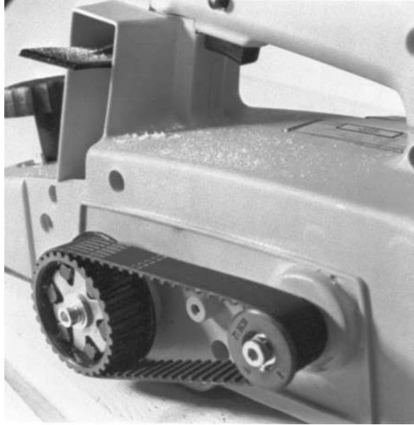
FIGURE 14.28 Planer machine drive with Synchrobel timing belt; the driving speed is 30\,000\text{ min}^{-1} . ( Continental Gummi-Werke Aktiengesellschaft. )
