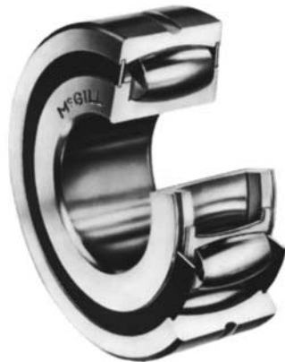
FIGURE 18.3 Rolling bearing with spherical rolling elements to permit misalignment up to \pm 3^\circ with an unsealed design. The sealed bearing, shown above, permits misalignment to \pm 2^\circ . ( McGill Manufacturing Company, Inc. )
