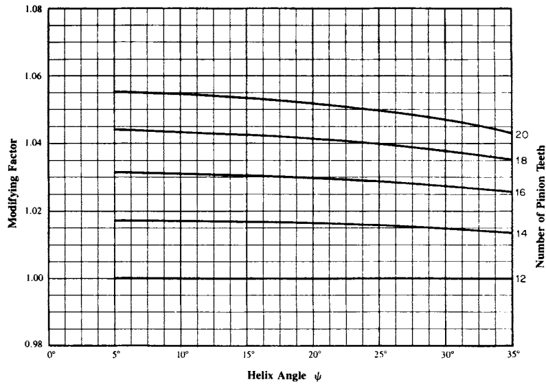
FIGURE 10.36 J factor multipliers for 20° normal-pressure-angle helical gears with short addendum (75 percent of standard). These factors can be applied to the J factor when other than 75 teeth are used in the mating element. (From Ref. [10.1].)
