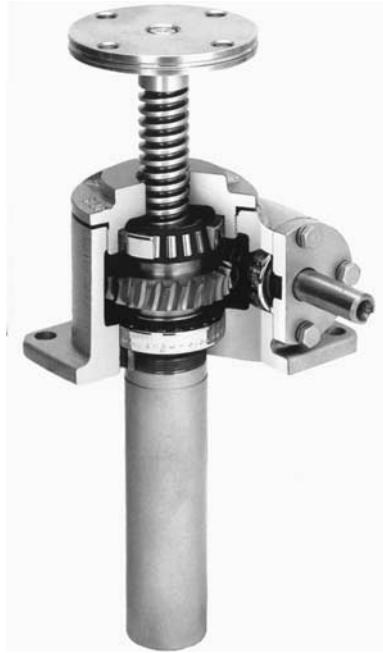
FIGURE 13.1 Power screw assembly using rolled thread load screw driven by worm shaft and gear nut. ( Simplex Uni-Lift catalog UC-101, Templeton, Kenly & Co., Inc., Broadview, Ill., with permission. )
