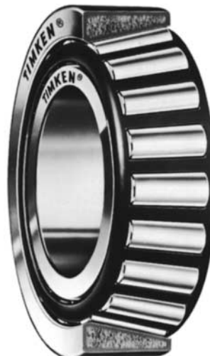
FIGURE 18.10 Tapered-roller bearing; for axial loads, thrust loads, or combined axial and thrust loads. (The Timken Company.)
