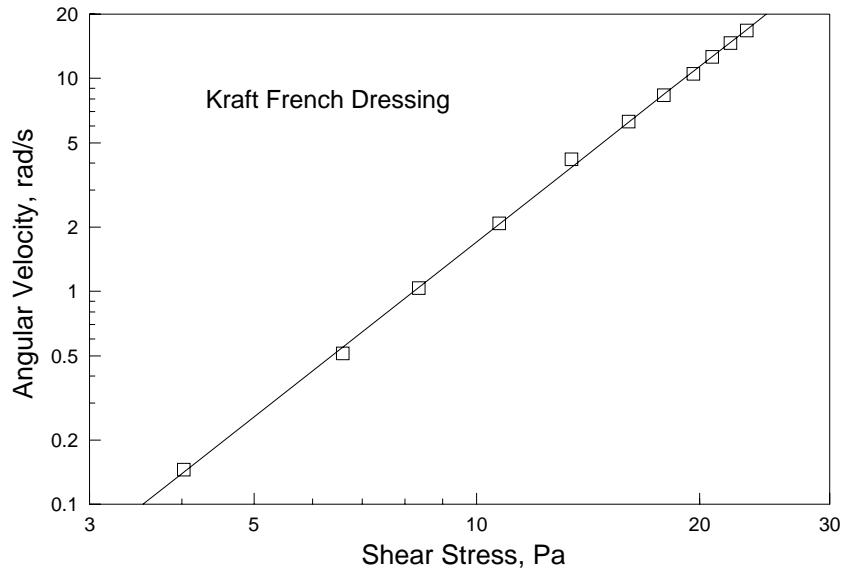
Figure 3.25. Logarithmic plot of angular velocity versus shear stress for Kraft French salad dressing.
